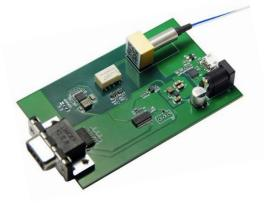
Agiltron offers Fiber Optic MEMS Tunable Filters with central wavelengths of 1060nm, 1310nm, 1550nm, and 2000nm. It is tunable continuously over a spectral range of up to 80nm at a speed of about 80ms. The wavelength tuning is actuated by driving a rotating MEMS mirror that is optically coupled with a grating and a dual fiber collimator. It is conveniently controlled with a user-friendly GUI and USB or RS232 and I2C control interfaces.
